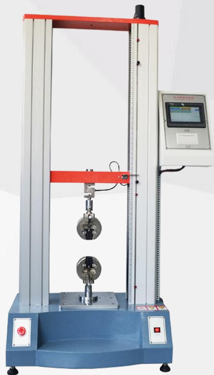
ZL-8002A Touch Screen Double Column Tensile Tester
